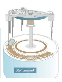
SC-120 supports the globally common stain protocols including Wright stain, Wright-Giemsa stain and May-Grunwald-Giemsa stain. The stain A could be recycled up to 20 times, this saves over 50% the stain compared to the conventional technologies.
