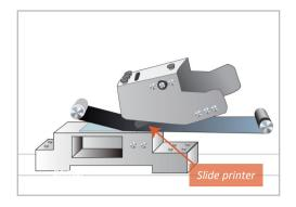
All patient information, including 1D or 2D barcode, number, as well as text could be printed on the frosted glass area of the slide with a durable thermal printer.
