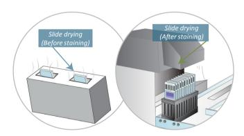
All slides are heat dried before and after staining. This optimizes staining quality and reduces contamination risk for the users.
