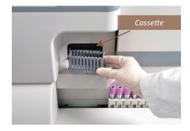
The cassette, which is used for carrying glass slides could be easily loaded from the front of SC-120, and be automatically transported inside by the track.
