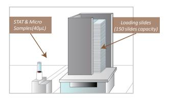
The STAT position ensures a faster blood smear preparation. This position can handle micro-samples requiring only 40µL blood, this is the smallest blood requirement in the hematology industry. Users are able to load up to 150 slides at a time into SC-120 for reducing the turn around time.
