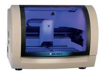
The **BD MAX™ System** for molecular diagnostics is the next generation platform which fully automates cell lysis, nucleic acid extraction, PCR set-up, amplification and detection.
